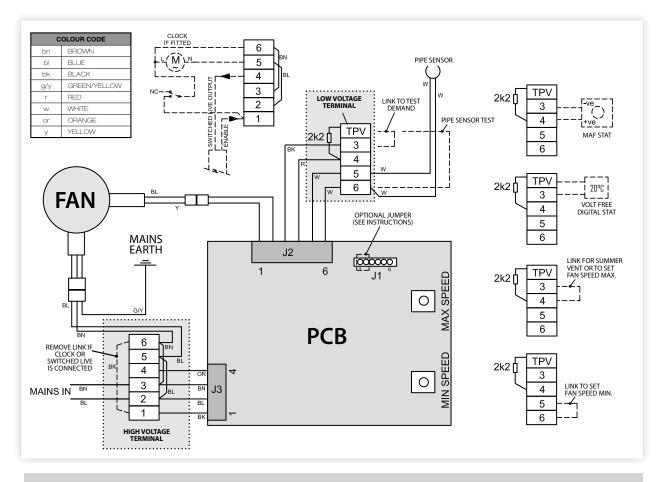
FIGURE 4. AQUAIR S CIRCUIT DIAGRAM
