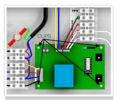
FIGURE 4. AQUAIR S PCB REMOVAL
