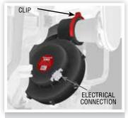
FIGURE 31. FAN REMOVAL
