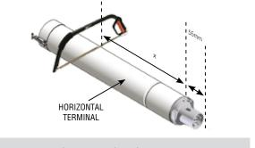
FIGURE 15. MEASURING THE FLUE
