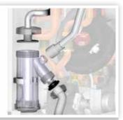
FIGURE 32. CONDENSATE TRAP
