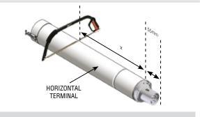
FIGURE 15. MEASURING THE FLUE
