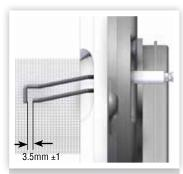
FIGURE 36. ELECTRODE GAP
