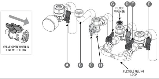
FIGURE 25. VALVES, TAIL PIPES & CONNECTIONS
