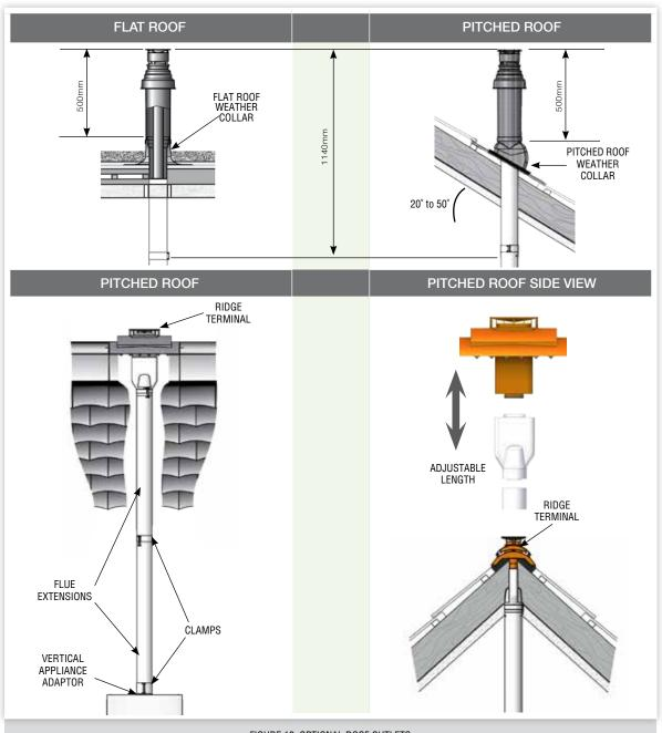
FIGURE 12. OPTIONAL ROOF OUTLETS
