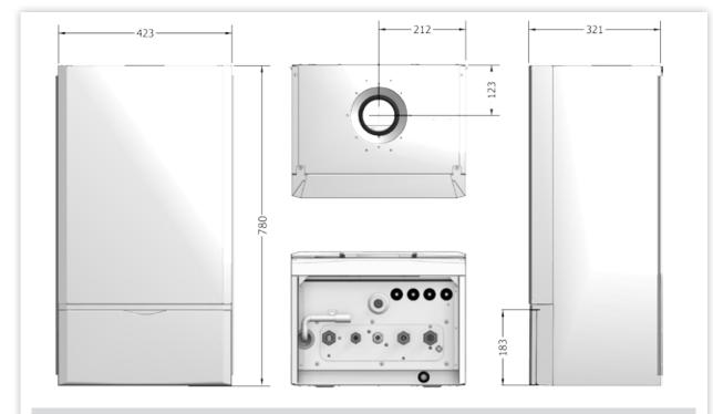
FIGURE 4. QUANTEC COMBI DIMENSIONS
