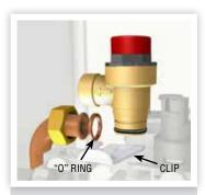
FIGURE 44. PRESSURE RELIEF VALVE
