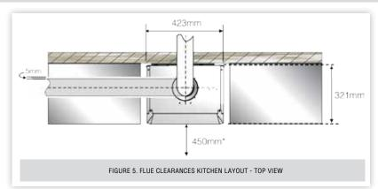
7.2.2 The minimum front clearance when built in to a cupboard is 5mm from the cupboard door but 450mm overall clearance is still required, with the cupboard door open, to allow for servicing.
