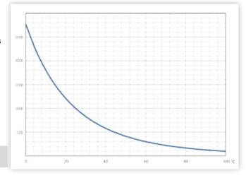
FIGURE 52. SENSOR TEMPERATURE/RESISTANCE DIAGRAM
