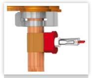
FIGURE 37. THERMISTOR SENSOR
