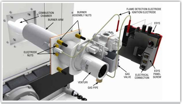
FIGURE 19. MAIN BURNER ASSEMBLY REMOVAL
