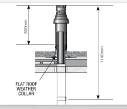
FIGURE 8. OPTIONAL ROOF OUTLETS
