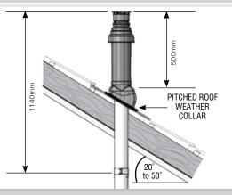
FIGURE 9. OPTIONAL ROOF OUTLETS
