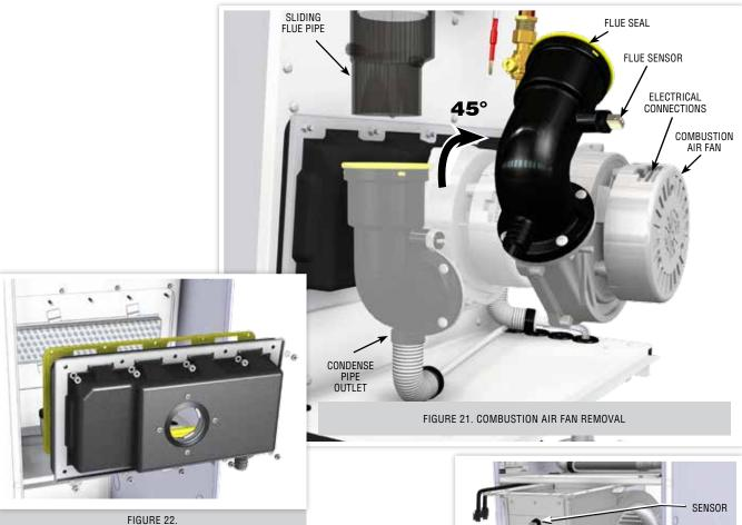
COMBUSTION AIR PASSAGE REMOVAL
