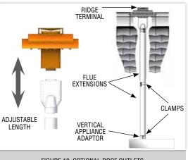
FIGURE 10. OPTIONAL ROOF OUTLETS
