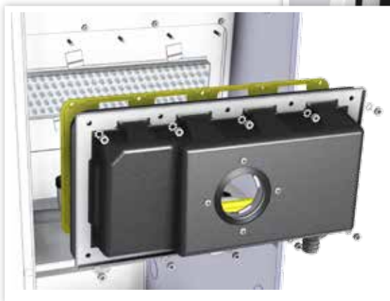
FIGURE 22. COMBUSTION AIR PASSAGE REMOVAL
