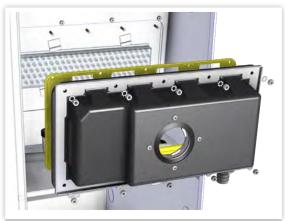
FIGURE 21. COMBUSTION AIR PASSAGE REMOVAL
