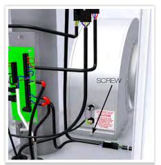
FIGURE 26. AIR CIRCULATION FAN ASSEMBLY
