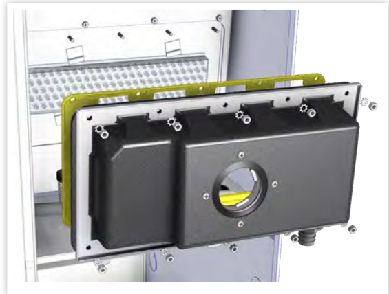
FIGURE 21. COMBUSTION AIR PASSAGE REMOVAL
