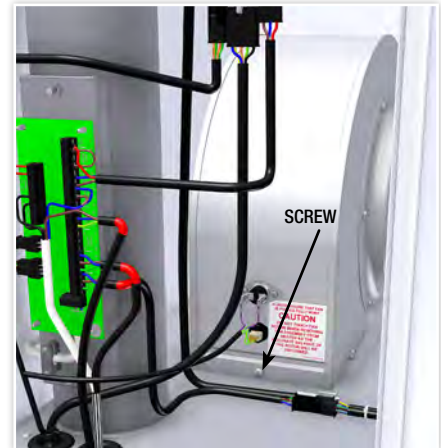
FIGURE 26. AIR CIRCULATION FAN ASSEMBLY
