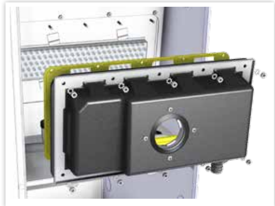
FIGURE 21. COMBUSTION AIR PASSAGE REMOVAL
