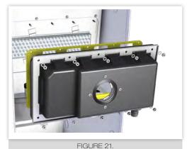
COMBUSTION AIR PASSAGE REMOVAL
